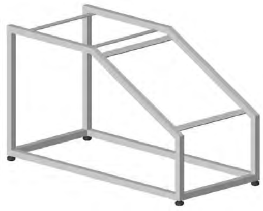
Shoe Fitting Stool Frame. Made from square stainless steel tube and bar.
